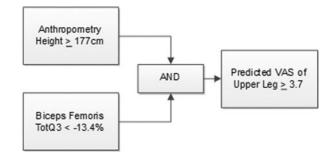
Figure 2. Sample use of a discomfort model. TotQ3, change in total blood volume in the third quarter. The threshold values were median values from the cross-validated data. Based upon the dichotomised data, if a person is taller than 177 cm and their total blood volume in the biceps femoris has dropped by 13.4% or more during the 60-90 min time window, then they are most likely to report a VAS score in the upper leg > 3.7 cm.
