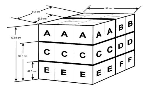
Figure 1. A schematic view of the six regions of the pallet.
