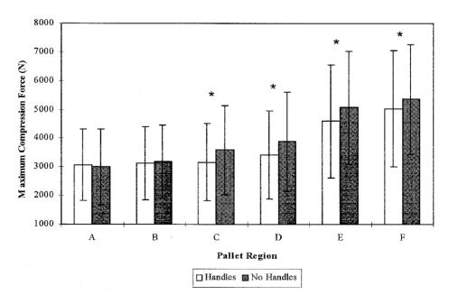
Figure 6. Maximum compression force as a function of handle coupling and pallet region (\* indicates a significant difference between the hand couplings).
